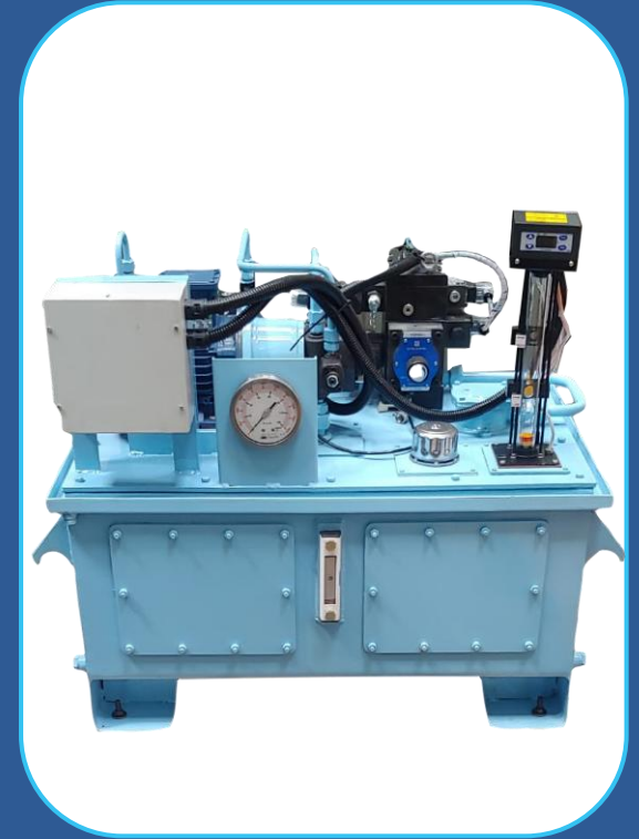
HYDRAULIC SYSTEM WITH TOWER BLOCK
